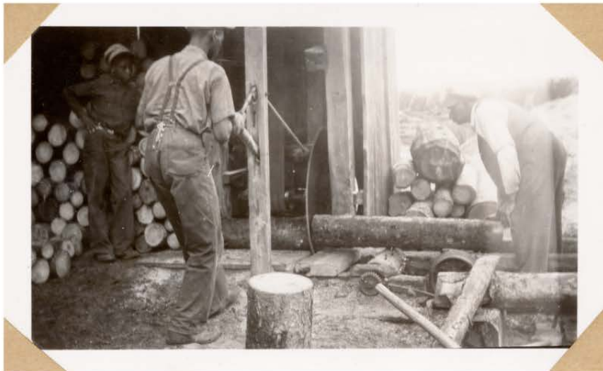
Cutting chunks. Note the mechanism for moving the circular saw back and forth; the young man in the center is operating it as Mr. Anderson moves the log forward. Note the roller under the log also, in order to move it forward easily.
